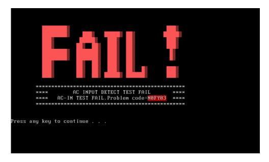
If it fails in a test item, press "Ctrl+C" and "Y" back to main menu.
